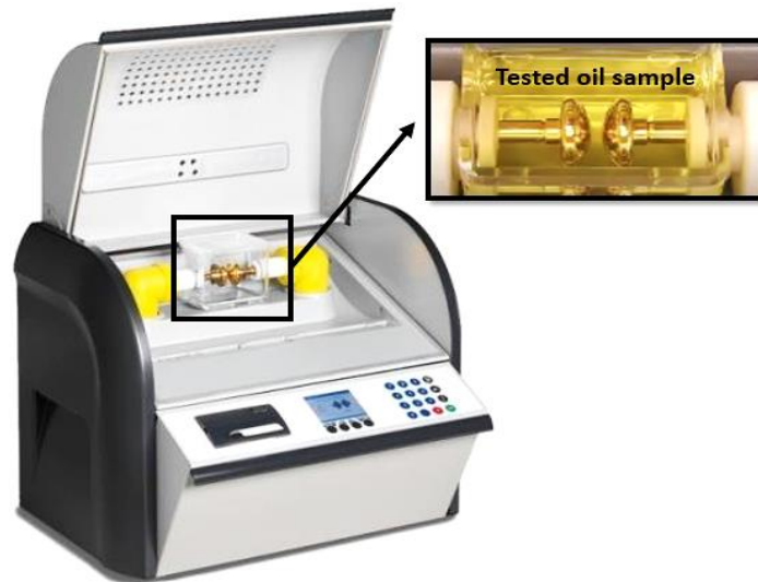
Figure 2. AC breakdown tester for liquid insulations.
